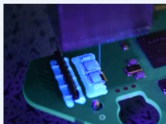
Low Pressure Jetting
